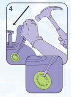
Put on protective gloves and goggles. Using a hammer and flat-head screwdriver, puncture the side of the small relief disc (D) on the back shoulder and pry open. You may have to puncture the ring in a few places around the disc to fully remove.
