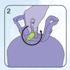
Remove the tilt nozzle (C) by turning the white valve nut counter- clockwise.
