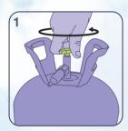
Fully open the valve (A) by turning counter-clockwise until it stops. Push down on the tilt nozzle (B) until hissing sound stops to release residual pressure. Ensure it is facing away from you.
