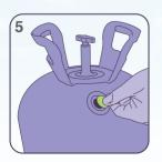
Remove the disc by hand. Edges may be sharp, wear gloves and use caution.
