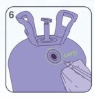
Circle the open hole and write EMPTY directly on the tank. Dispose of the other recyclables.
